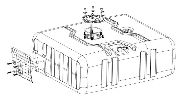
(Fig. 3) Exploded view showing the assembly of TITAN<sup>™</sup> model 8020199 replacement tank. Grounding Cable is <u>not</u> shown. The metal side shield is transferred from the OEM tank if it is so equipped.
