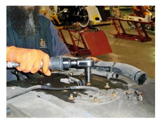
(Fig. 1) Loosen the bolts holding the sending unit into the OEM tank.
