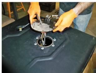
(Fig. 2) Carefully place the OEM sending unit into the new TITAN<sup>™</sup> replacement tank.
