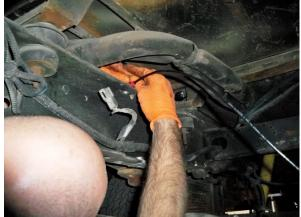
(Fig. 4) Be sure to attach Grounding Wire to one of the studs holding the sending unit.
